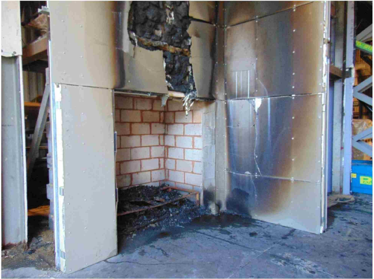
Figure 26. Post-test view of panels adjacent to combustion chamber.
